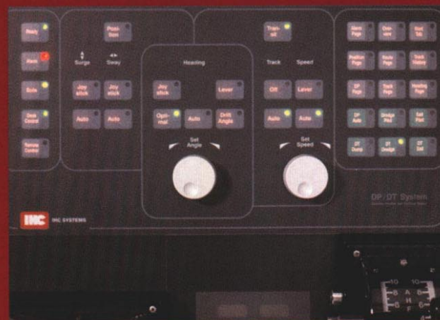
Fig. 5: Simple operation by 2 knobs for heading (left) and speed (right)
